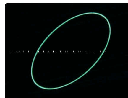
Fig. 3: This indicates a phase angle of around 55° (see text).
