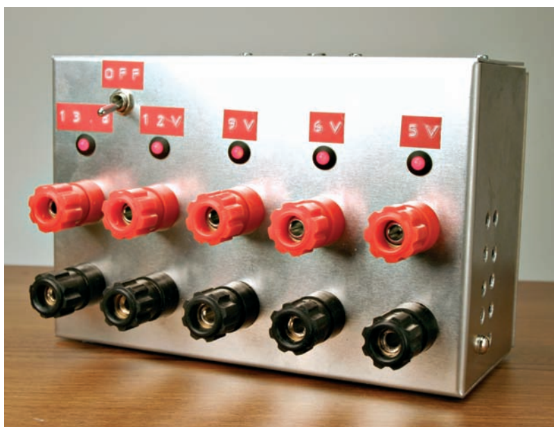
● Fig. 3: Note the ventilation holes down both sides of the case (and heading photo). These are needed to allow the heat, generated within the unit, to escape.
